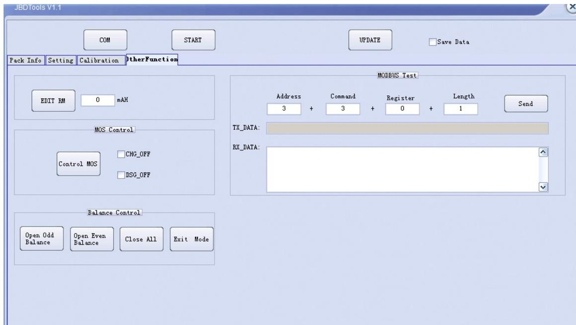
Mainly contains some test functions: edit the remaining capacity, control MOS tube, balanced test function, and MODBUS protocol debugging tools.
