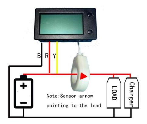
When the measured voltage range is over DC5 $\sim$ 90V, we should look for another power supply for <u>Coulometer</u>. As follows:
