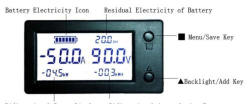
Bidirectional Power Display Bidirectional Accumulative Energy
